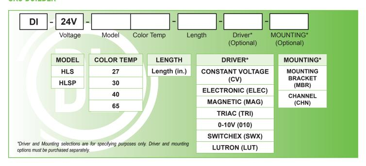
Example: DI-24V-HLSP30-384-ELEC-CHN = Diode, 24 Volt, HYDROLUME® SLIM HD, 3,000° CCT, 384 in. (32 feet), with Electronic Driver, and Mounting Channel
